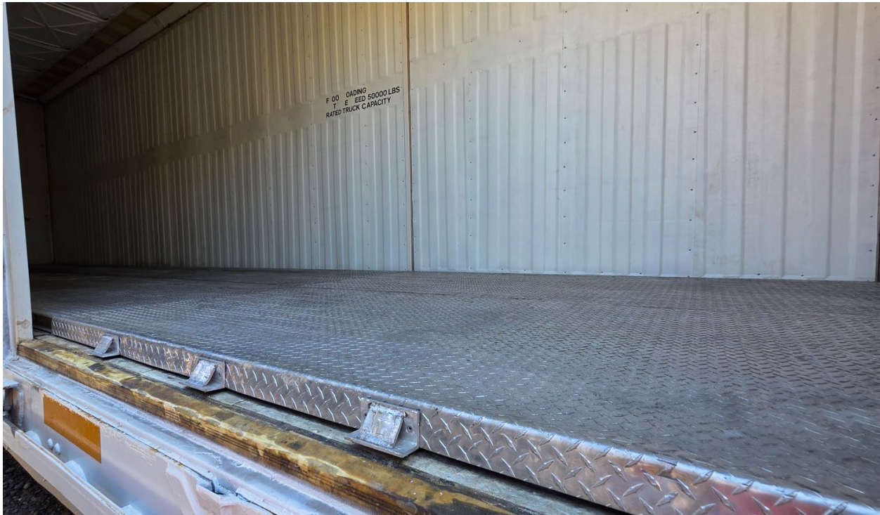
Exhibit C: Plastic wall panels and diamond plate floor.
